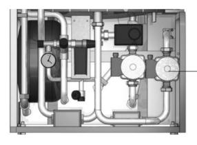
\_ Heat carrier pump (290 A/W)
